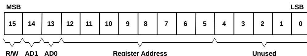
Figure 5. Bit Assignment and Definition for Slot-0 Word
